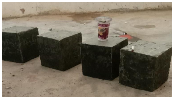
Figure 2.1 Cube test object (15 x 15 x 15) cm
