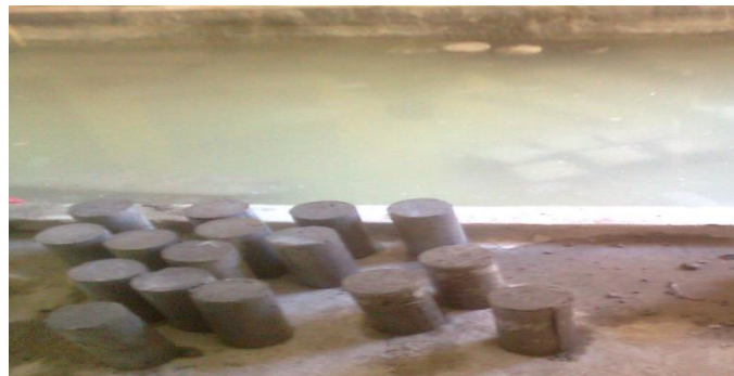
Figure 2.4 Cylindrical specimen (15 x 30) cm surface dry
