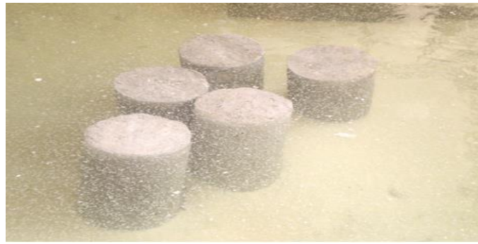
Figure 2.3 Treatment of cylindrical specimens (15 x 30) cm
