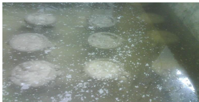
Figure 2.2 Cylindrical specimen (15 x 30) cm after casting in brackish water
