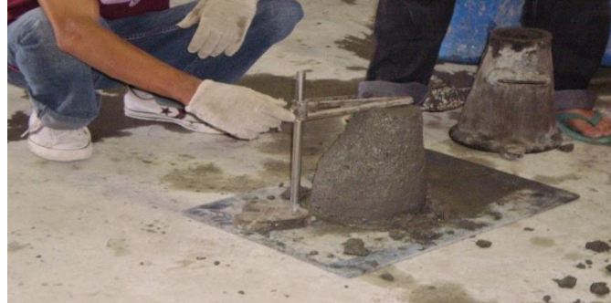
Figure 3.1 Slump value measurement
