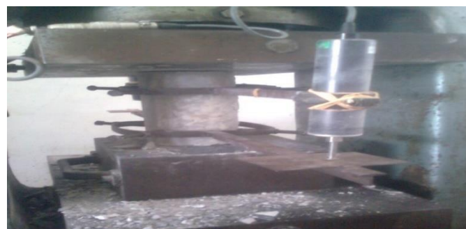
Figure 2.6 Testing the compressive strength of a cylindrical specimen (15 x 30) cm
