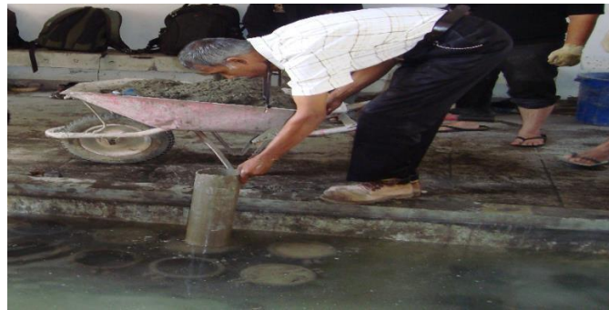
Figure 2.1 Method of casting in brackish water
