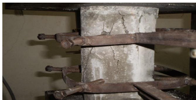
Figure 2.8 Cylindrical specimen (15 x 30) cm after testing
