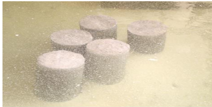
Figure 2.3 Treatment of cylindrical specimens (15 x 30) cm
