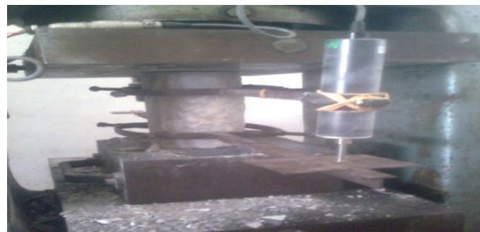
Figure 2.6 Testing the compressive strength of a cylindrical specimen (15 x 30) cm
