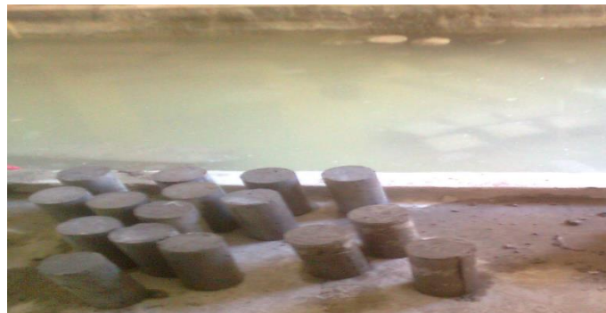
Figure 2.4 Cylindrical specimen (15 x 30) cm surface dry
