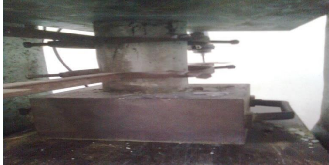
Figure 2.7 Cylindrical test object (15 x 30) cm after testing
