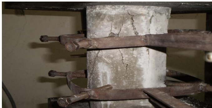
Figure 2.8 Cylindrical specimen (15 x 30) cm after testing
