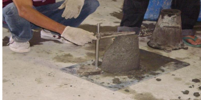
Figure 3.1 Slump value measurement
