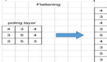
From the pooling layer (on the left) from the previous process, we simply take each row and combine them into one column. The first row (4, 3, 4) is combined with the second row (3, 5, 4) and then the third row (3, 5, 3). After we perform flattening, we input the results into the input layer of an ANN. The display is as follows:
