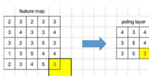
f. Flattening: The flattening stage converts the matrix in the pooling layer into a single column (a single vector). This vector will then become part of the input layer in an artificial neural network (ANN).
