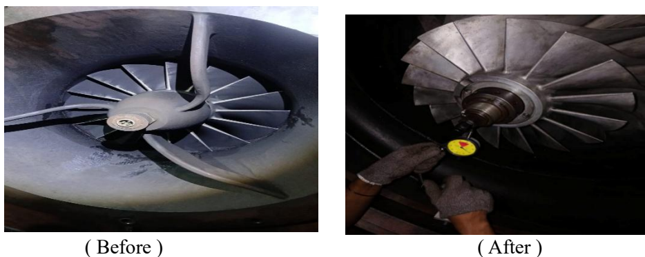
Figure 3.2 Before and After Turbocharger Maintenance
